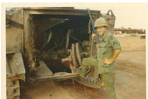
Damaged M113.JPG | M113 that was damaged by an RPG during an ambush. (Thanks to Tom Petro for the recollections.) (992x688)
